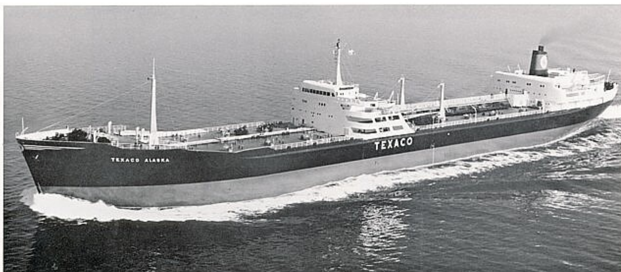
S.T. TEXACO ALASKA, turbine tank ship 41,050 tons d.w., 17¼ knots.
