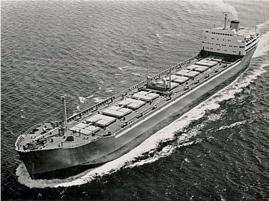
Virtala , motor ore and oil carrier, 21,900 tons d.w., 7,200 b.h.p., 14.5 knots, built for Trafikaktiebolaget Grängesberg—Oxelösund, Stockholm.
